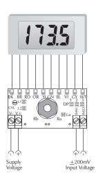
Measuring a floating voltage source of 200mV full scale. Add Ra and Rb and cut Link La to increase the measurement range.
