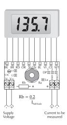
Measuring current. Recalibrate the module. The current to be measured must be isolated from the module's power supply.
