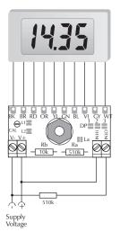
Measuring a supply voltage. (min. 7.5V, max. 15V) Cut Links La and L2. Recalibrate the module.
